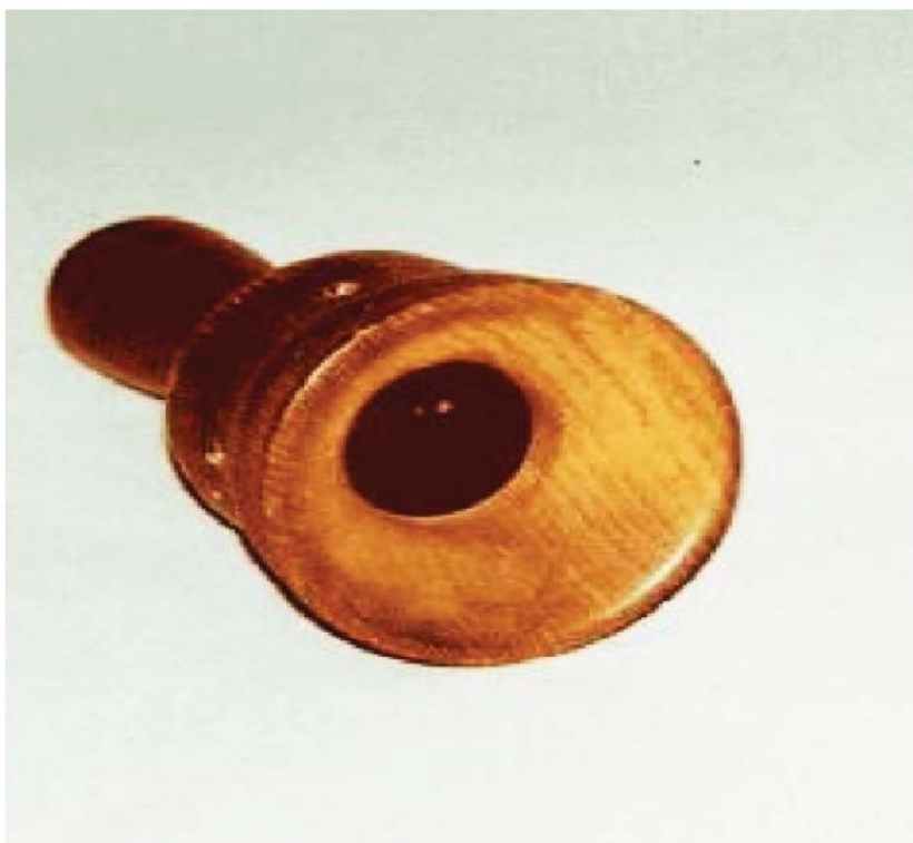
Fig. 9. Marconi's reconstruction of Meucci's 1857-67 Telephone. (Photo by Maurizio Ghisellini for Basilio Cantania in the early 1990's).
